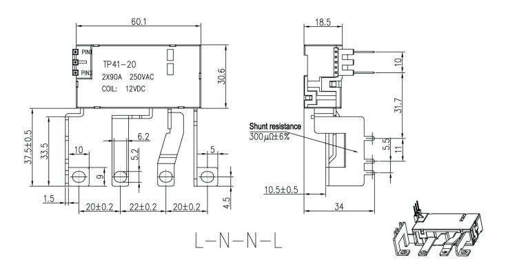
Remark: The tolerance didn't mark on drawings. When dimension is  $\leq$  1mm, the tolerance should be less than  $\pm$ 0. 2mm; when dimension is between 1-5mm, the tolerance should be less than  $\pm$ 0. 3mm; When dimension is  $\geq$ 5mm, the tolerance should be less than  $\pm$ 0. 5mm.
